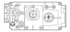
**Note:** Knob cannot be turned from "PILOT" to "OFF" unless the knob is pushed in slightly. Do not force.
